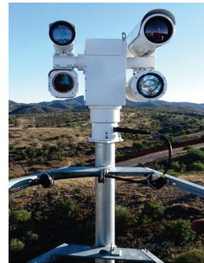
*Cameras mounted atop a Remote Video Surveillance System (RVSS) tower in Texas.*
